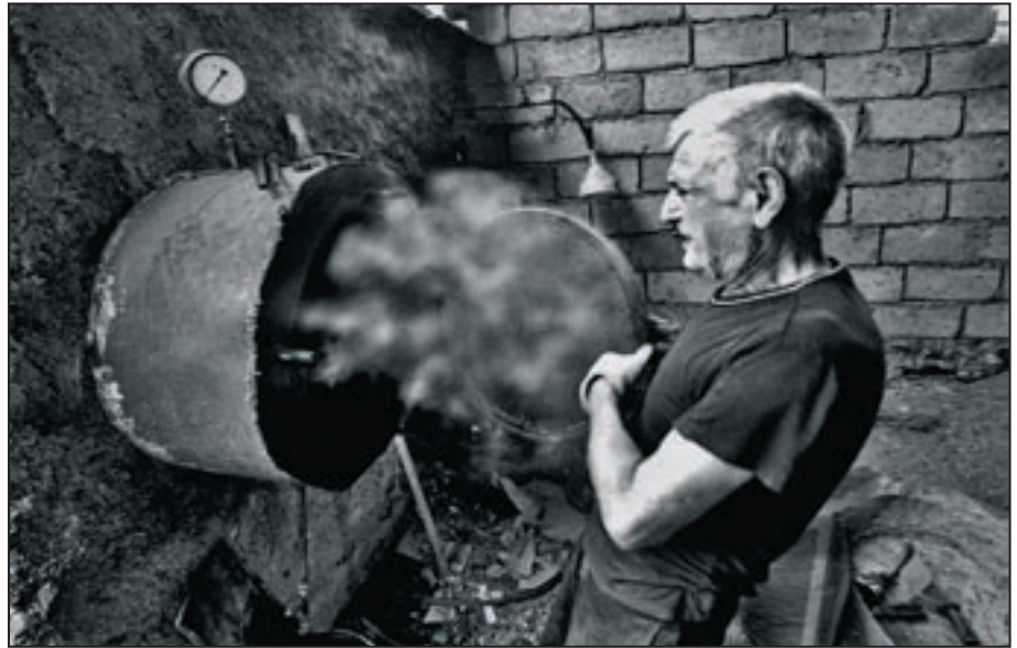
↑ The boards soften nicely in the steam.
